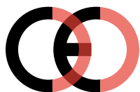
False CE Mark (too close)
