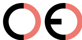
False CE Mark (too far)
